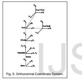
A 6DOF robot arm modeling was discussed as an example in the present work. The basic kinematic model of the robotic arm is shown in Figure 4. DH mechanism works with quadruple (1), which represents twist angle, link length, link offset and joint angle respectively. The pictorial representation of DH convention method of the manipulator in an orthonormal coordinate system is shown in Figure 5.
